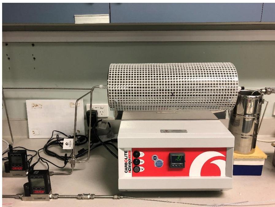
Figure 3.18 Temperature programmed reduction apparatus
